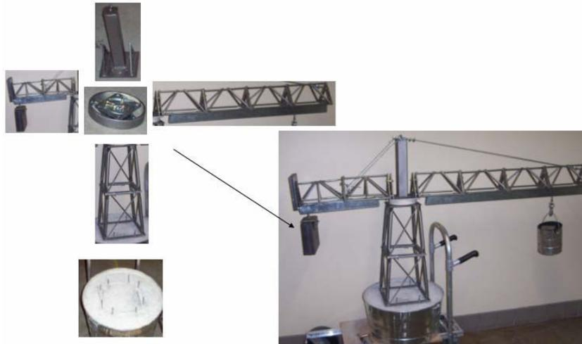
Figure 4. Roof panel lift mechanism
