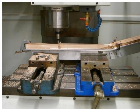
**Figure 5: Hurco CNC milling machine cutting guitar neck**
