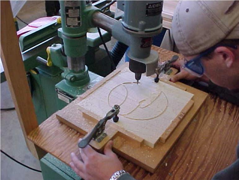
Figure 3: Manual pin routing using a CNC-machined jig
