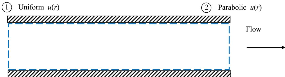
**Figure 6. Control volume selected to expose viscous frictional forces at the walls and pressure forces at the ends.**
