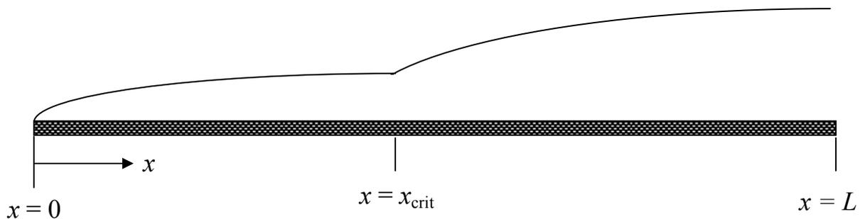
**Figure 8. Mixed laminar-turbulent boundary layer growing over a flat plate in a uniform flow.**
