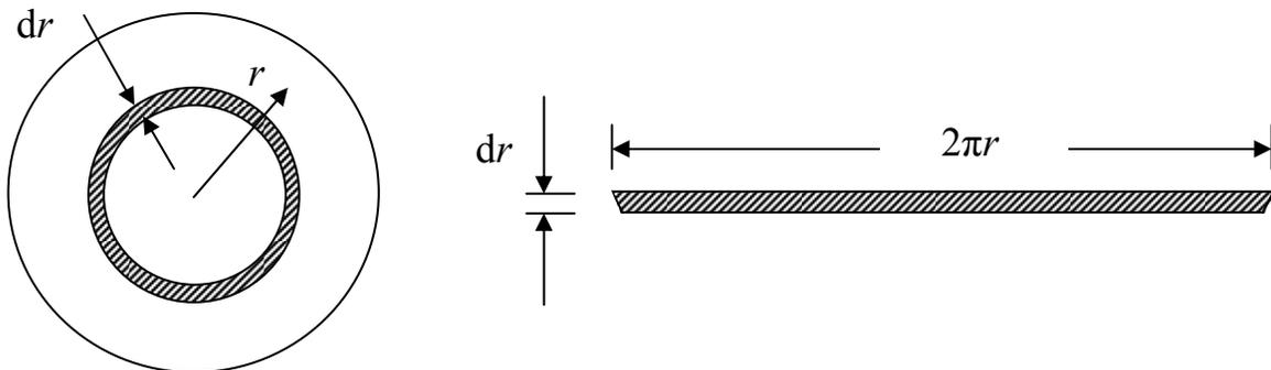
**Figure 3. Differential control volume for pipe flow.**
