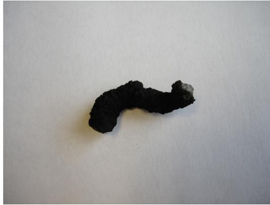
Figure 3. Typical carbon nanotube-rich deposit
