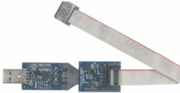
Figure 3: Silicon Laboratories Debug Adapter Daughter Card<sup>3</sup>
