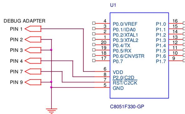
Figure 4: Programming the C8051F330-GP DIP Using the Debug Adapter
