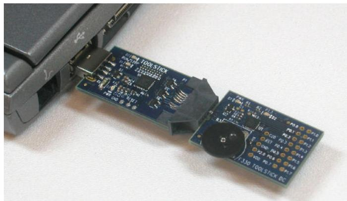
Figure 1: Silicon Laboratories USB ToolStick<sup>2</sup> (courtesy of Silicon Labs.)
