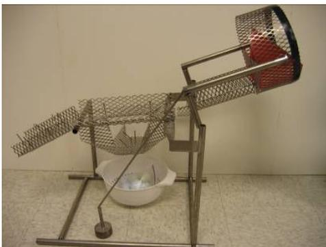
Figure 4: Gravity lifter, pachinko timer-sorter
