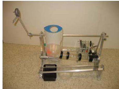
Figure 3: Gravity lifter, size sorter, electric timer
