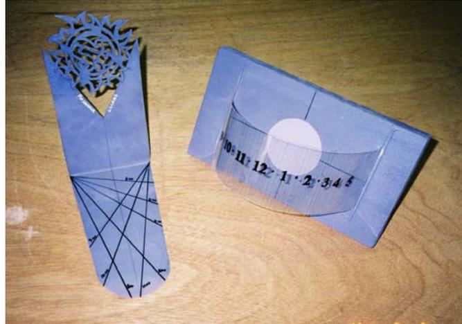
Figure 14: Interesting simple devices but both reversed AM and PM.
