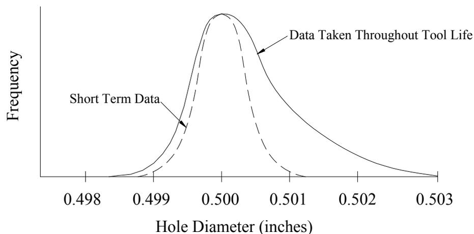
**Figure 1. Hole Diameter Distribution**
