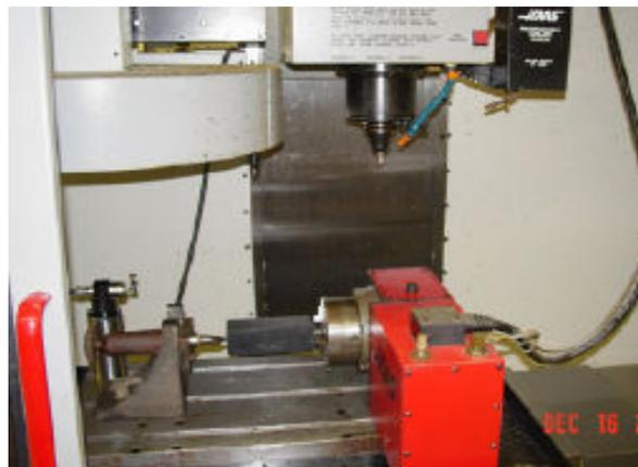
Figure 1: 4-axis HAAS VMC setup
