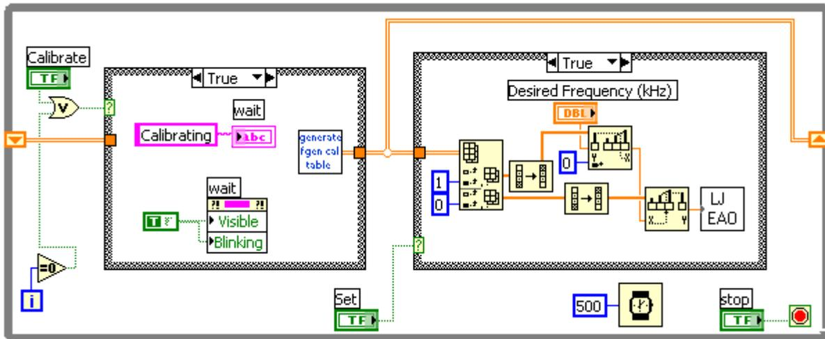
Figure 9. LabVIEW Diagram for Function Generator Example
