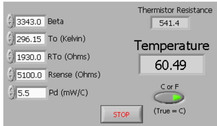
Figure 3. LabVIEW Front Panel for Thermistor Experiment
