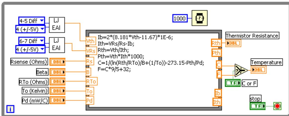
Figure 4. LabVIEW Block Diagram for Thermistor Experiment
