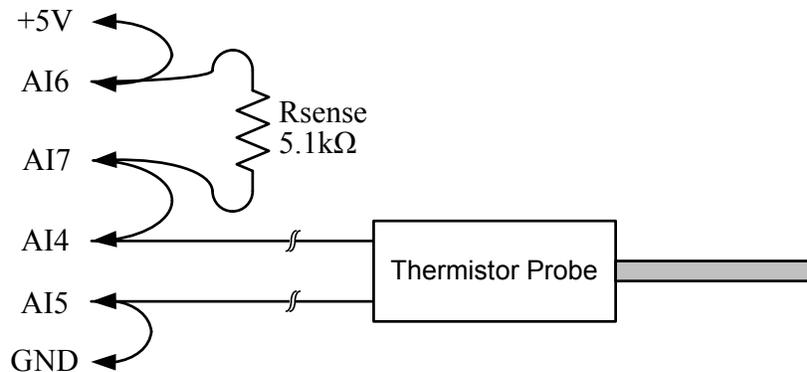
Figure 2. LabJack Wiring Diagram for Thermistor Experiment
