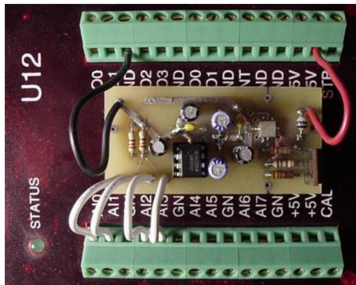
Figure 6. Accelerometer Circuit Board on LabJack
