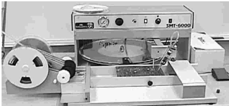
**Figure 4.** Manual X-Y arm assisted placement station.
