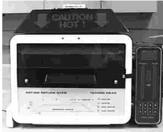
**Figure 3.** Batch reflow oven
